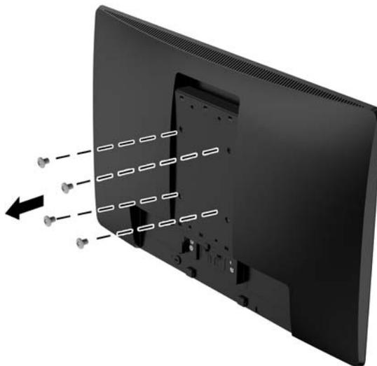
4. Secure the mounting plate to the wall or swing arm of your choice using the four screws included with the mounting plate.
